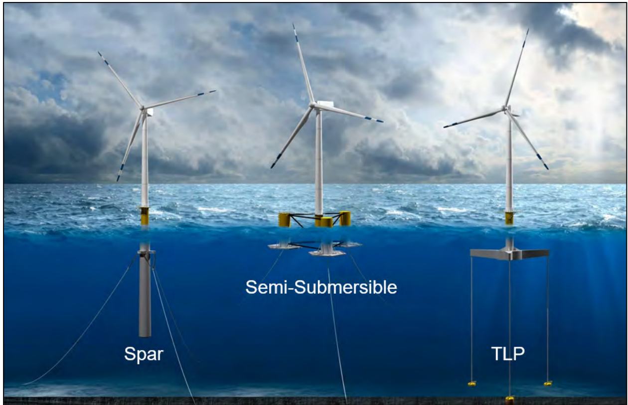
Figure 4.1. Illustration of floating foundation types (left to right: spar, semi-submersible, TLP) (NREL 2022)
