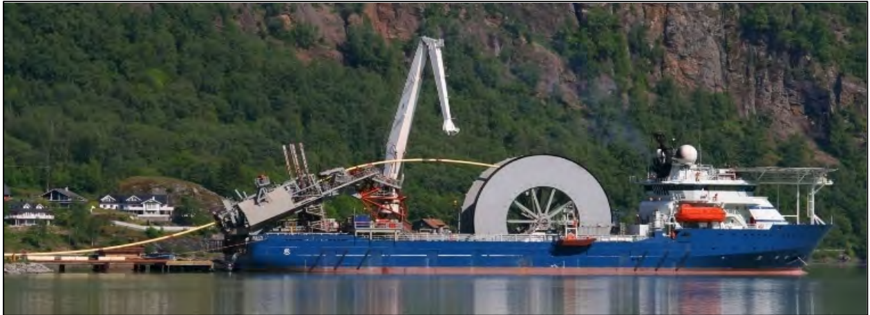
Figure 3.5. Cable laying vessel (Marine Insight 2021)
