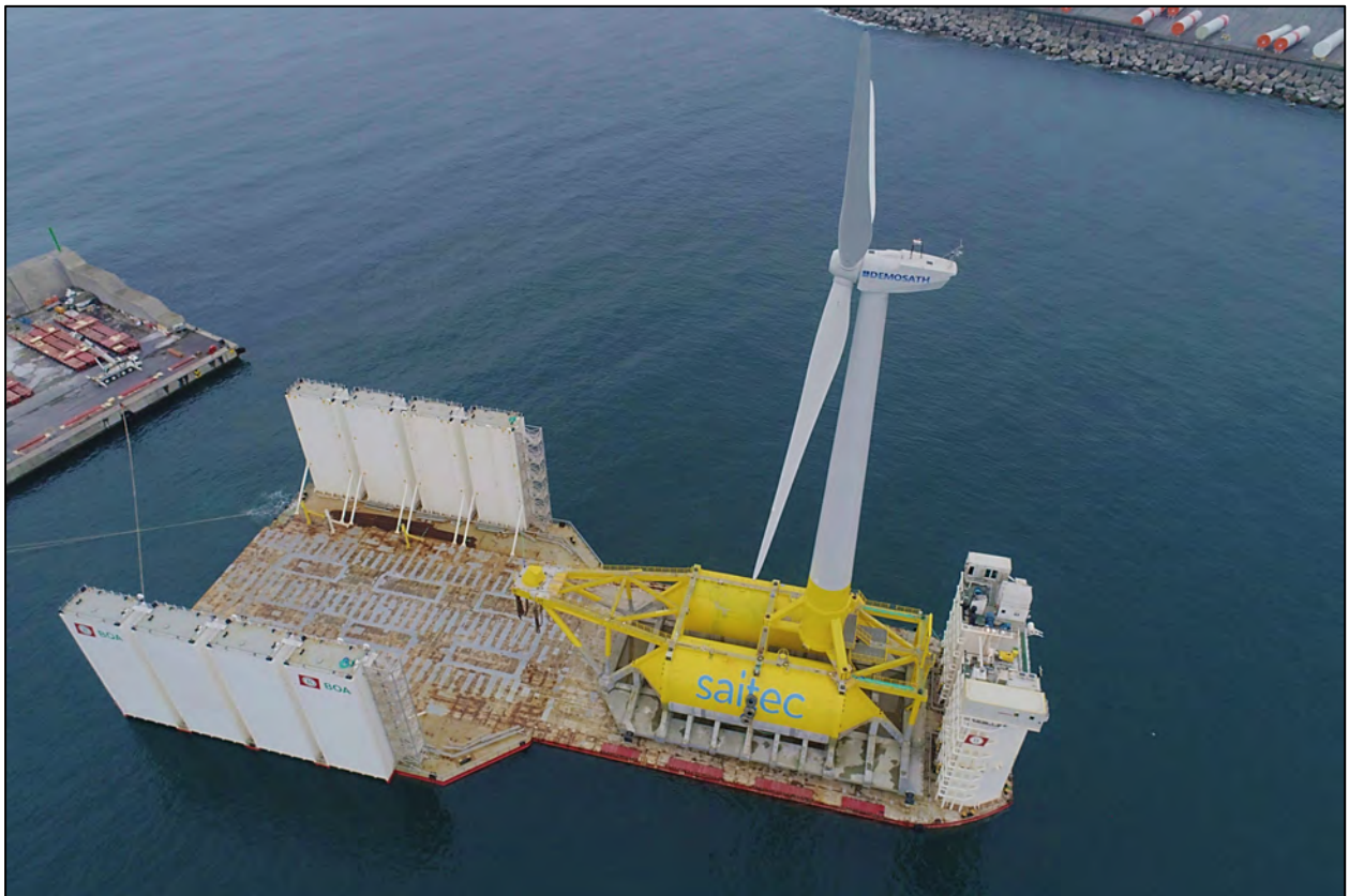
Figure 3.8. Semi-submersible barge (BOA 2022)
